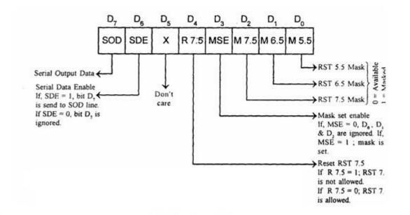
D7-D6 - The left two bits are related to the serial interface. When D6 (SDE-Serial Data Enable) is 1, then whatever is in D7 (SOD-Serial Data Output) is written to the serial data output (pin 4 of the 8085). If D6=0, nothing is written. This allows a SIM instruction to be executed altering interrupt masks without affecting serial data.
