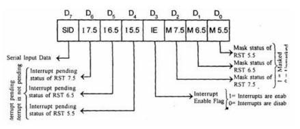
Bit D7 (SID-Serial Input Data) This is the input pin of the serial data interface which is connected to pin 5 of the 8085, and indicates the high/low status of that pin.
