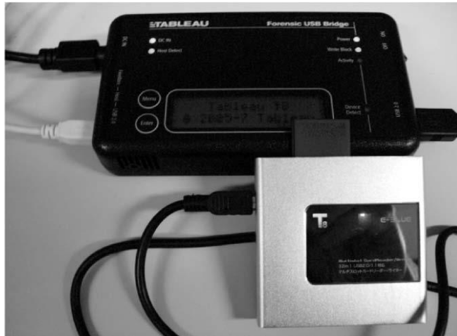
Figure 2.12.2 A multi-format removable memory card reader connected via a forensic bridge write-blocker
