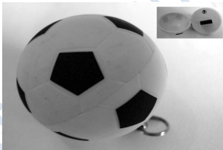
Figure 1.9.3 A novelty/disguised USB storage device (inset shows the USB connector visible when it is opened)
