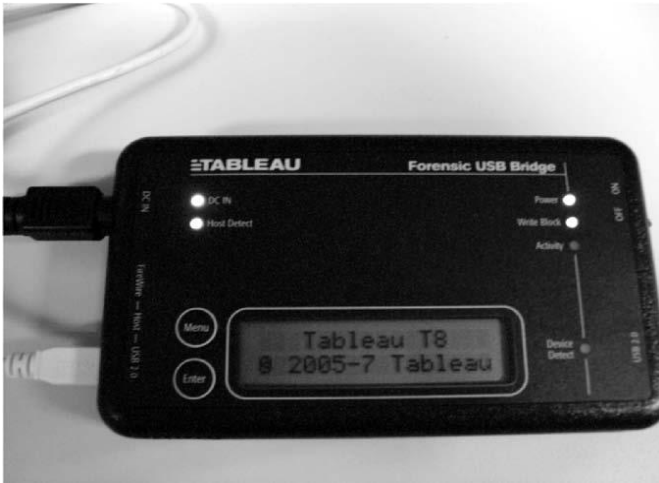
Figure 1.12.1 A Tableau T8 USB write-blocker used to protect devices against accidental data writing
