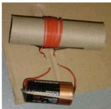
Figure 2. Setup for an Electromagnetic Field Station.
