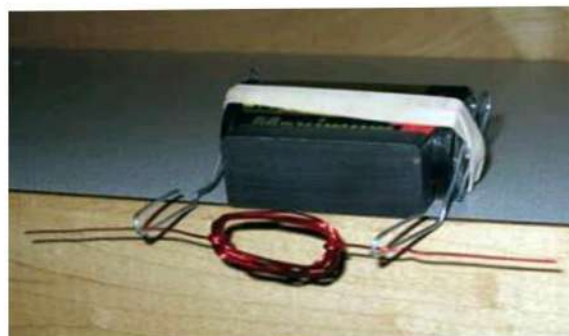
Figure 6. The complete motor setup.
